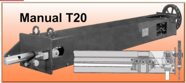
The Clyde Bergemann Model MT20 manual long retractable sootblower is designed for use in package boilers, small industrial boilers and oil fired heaters with travels of 10 feet of less. The MT20 uses a formed steel housing covering the top and sides, a 2 3/8" OD alloy steel lance, a 304 SS feed tube and wall sleeve mounted to the front support yoke. Operation may be by chain or hand crank. A manual medium admission valve must be supplied for installation in the inlet pipe.
